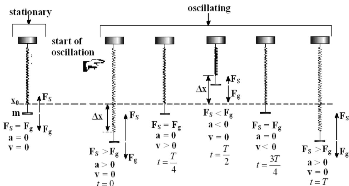
The oscillation will proceed with a characteristic period,  $T$ , which is determined by the spring constant and the total attached mass. The period is given by:
